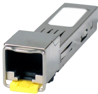
Figure 2.3. A typical 1000 Base TX module
