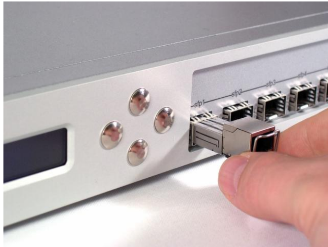
Figure 2.4. Installing a 1000 Base TX module
