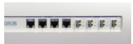
Clavister XC4080B with 4 copper and 4 fiber gigabit Ethernet interfaces.
